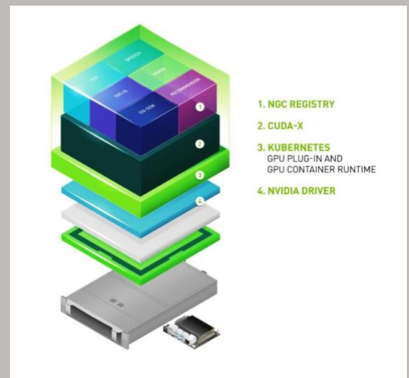
Figure 2 - NVIDIA's EGX Stack
