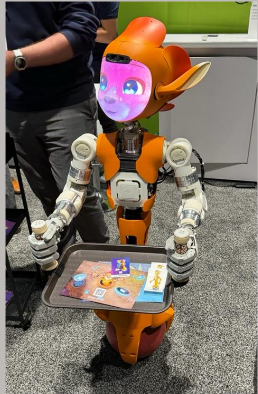
Humanoid Robot from Enchanted Tools using twin Jetson Orin platforms
